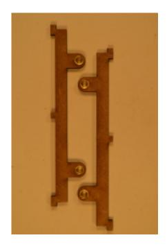
Assemble the 6 pieces as shown by locating the tabs on the 2 sole bar pieces into the the holes in the floor piece and the end pieces, ensuring that the flanges on the brass bearings are facing out, then fit the centre spacer.
