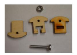
Locate the parts which make up the buffer. and glue all three sections together with the screw in the middle and the grooves on the outside pieces facing inwards to locate the screw head. Ensure that the small hole in all three parts line up so that the rod for the coupling can be passed through. Finally clamp all three sections untill the glue has set.
